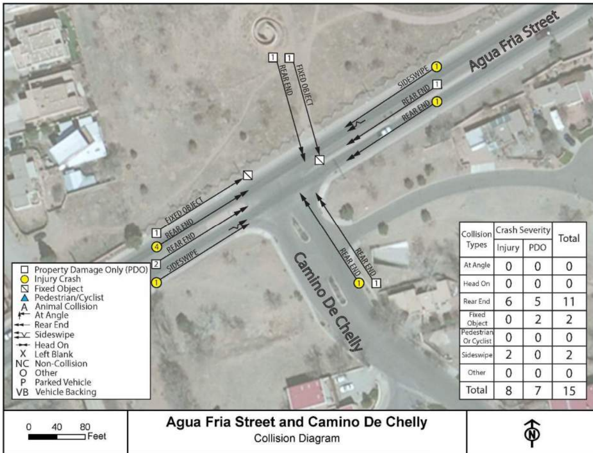
Figure 26: Intersection #9 – Agua Fria Street and Camino de Chelly – Crash Types and Crash Severity
