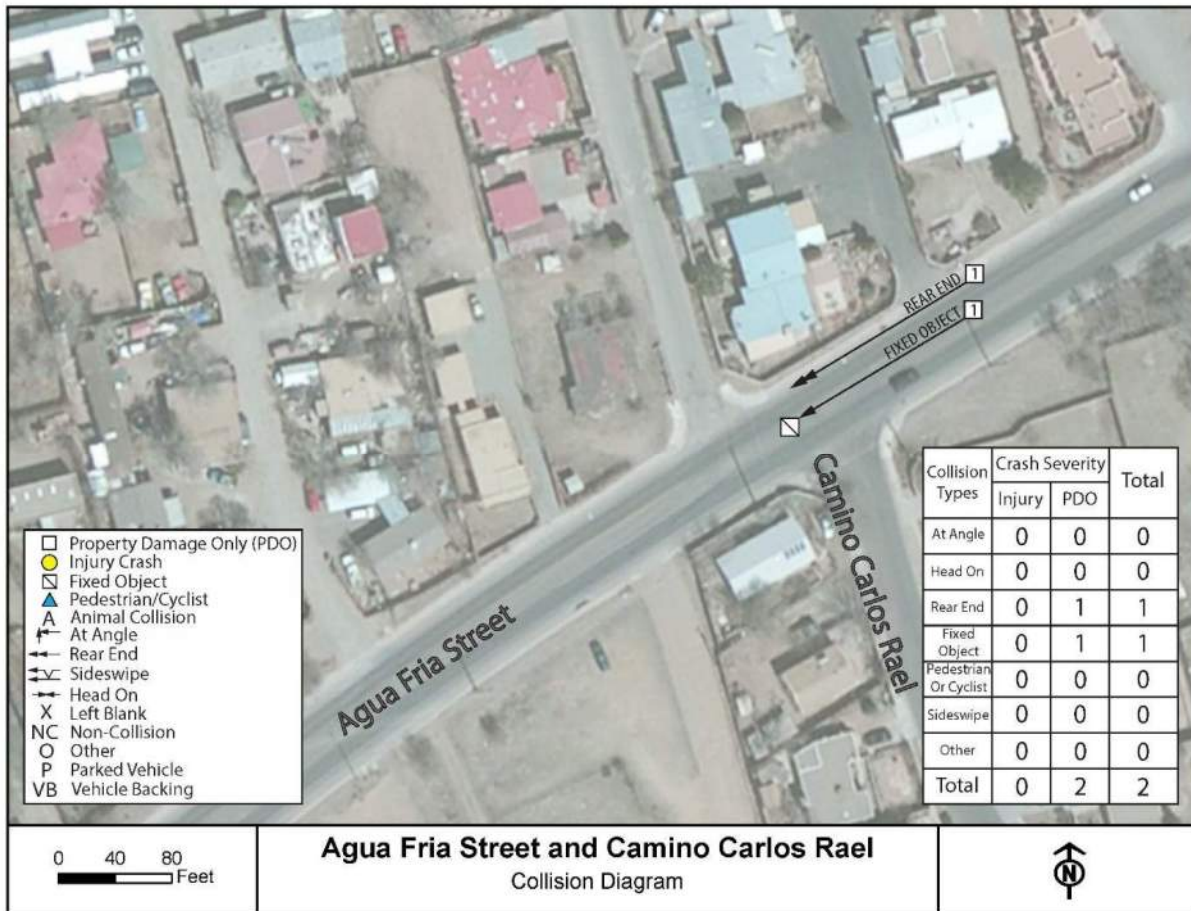
Figure 19: Intersection #6 – Agua Fria Street and Camino Carlos Rael – Crash Types and Crash Severity
