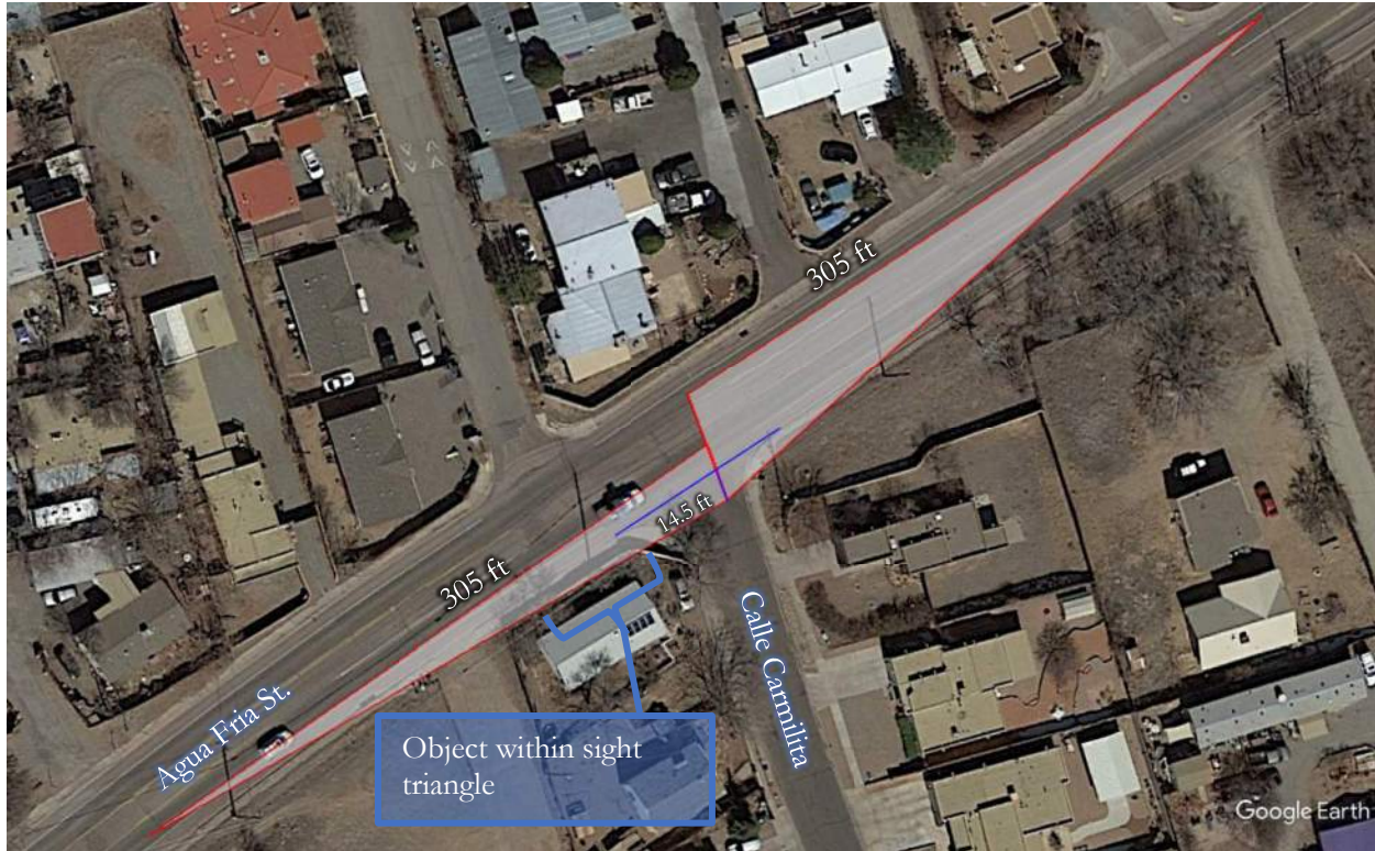
Figure 22: Intersection #7 – Agua Fria Street and Calle Carmilita. Northbound Approach Sight Distance
