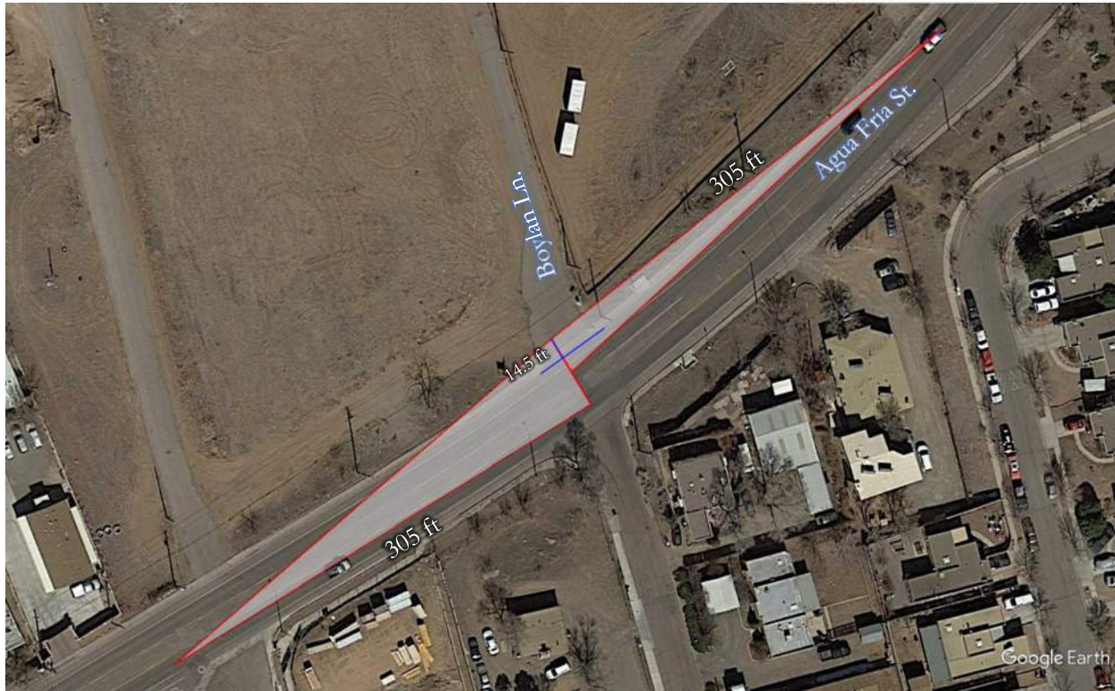
Figure 14: Intersection #3 – Agua Fria Street and Boylan Ln. Southbound Approach Sight Distance
