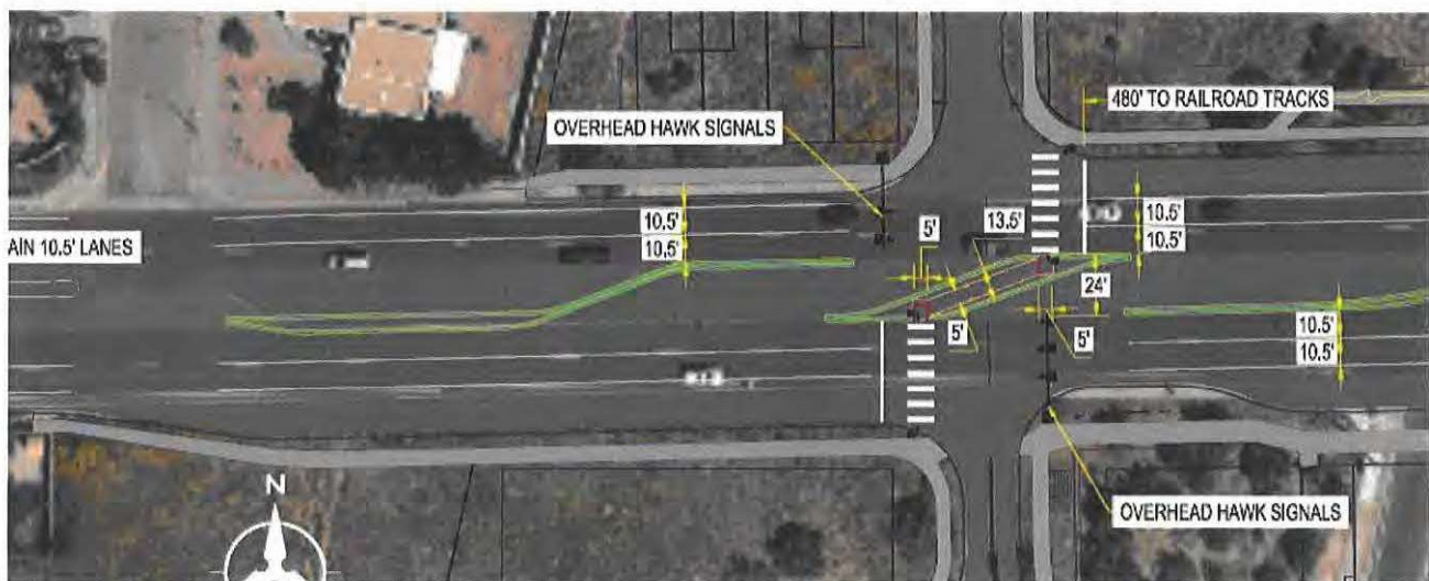
Proposed HAWK pedestrian crossing at realigned Galisteo Street, also showing U-turn accommodations just east of Galisteo, where the ROW is widened for a deceleration/right turn lane.
