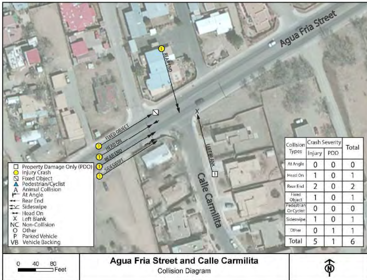
Figure 21: Intersection #7 – Agua Fria Street and Calle Carmilita – Crash Types and Crash Severity
