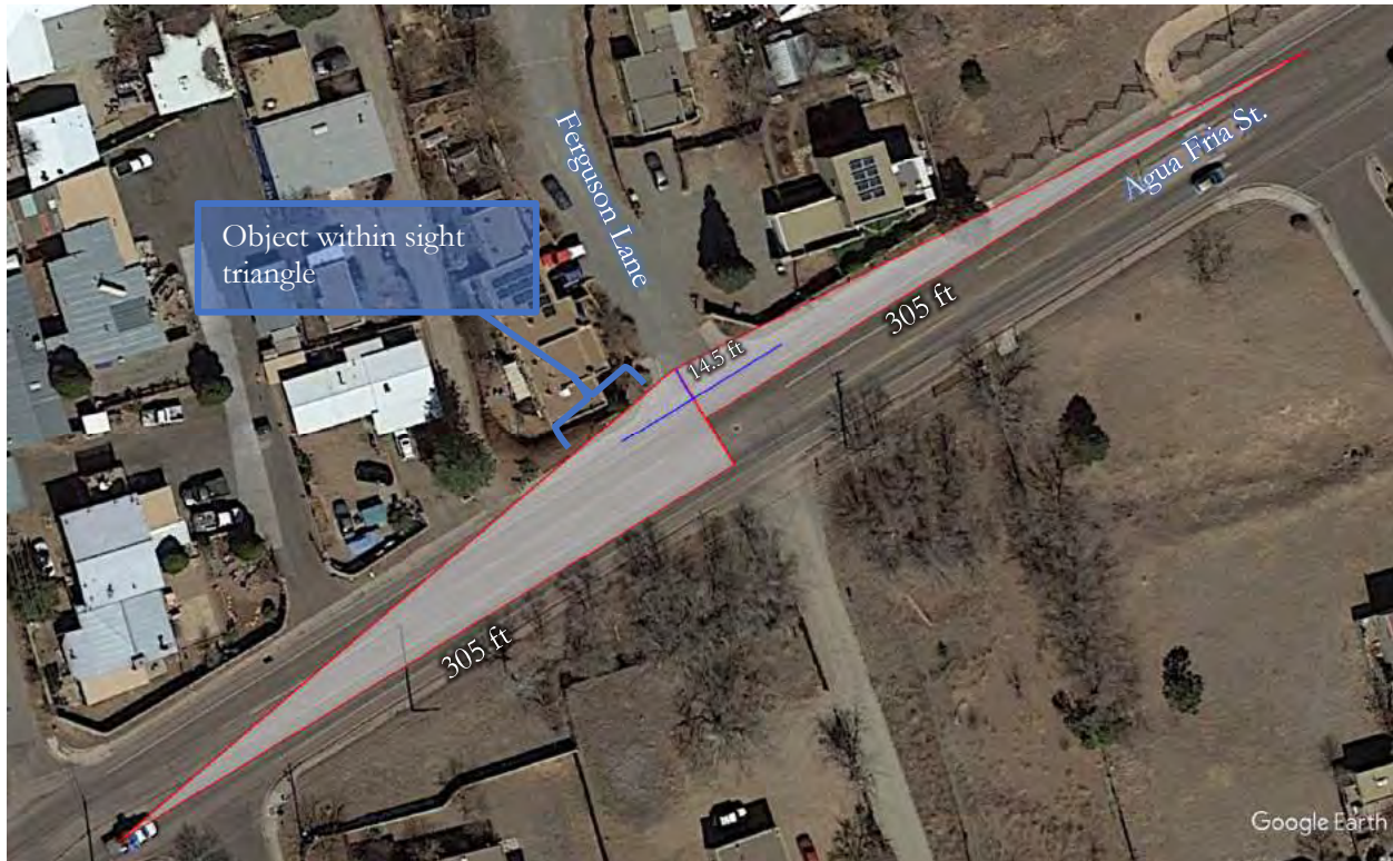
Figure 24: Intersection #8 – Agua Fria Street and Ferguson Lane Southbound Approach Sight Distance
