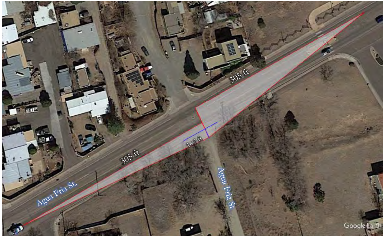
Figure 25: Intersection #8 – Agua Fria Street and Agua Fria Street Northbound Approach Sight Distance
