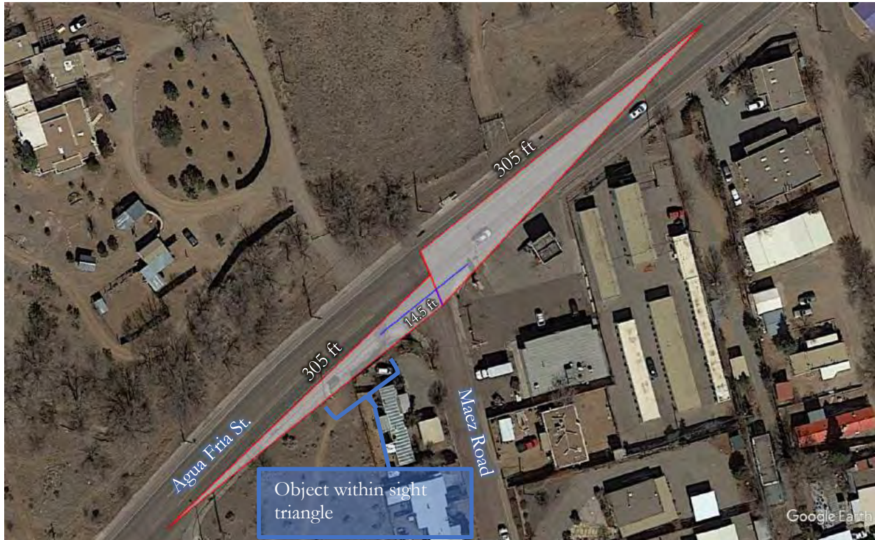
Figure 18: Intersection #5 – Agua Fria Street and Maez Road Northbound Approach Sight Distance
