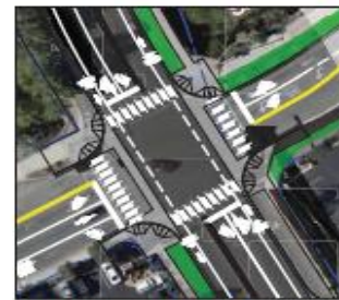
Eliminate EB Right-Turn Lane
