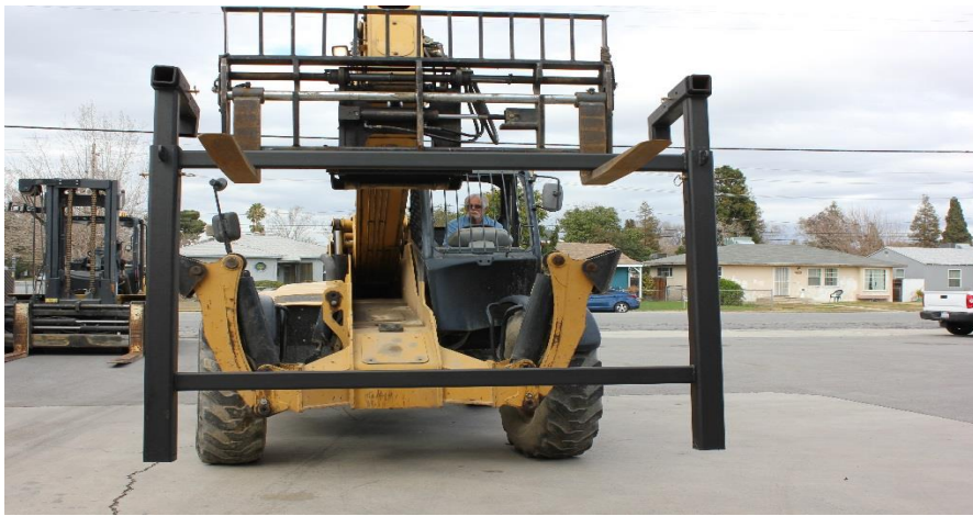
Lift Unit – 5 Parts: 1 Frame, 2 Vertical Extensions, 2 Horizontal Extensions
