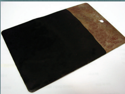
STRYK 5388 FACS® applied on Cold Rolled Metal Q-panel 10 Mils dried film thickness or Dft
