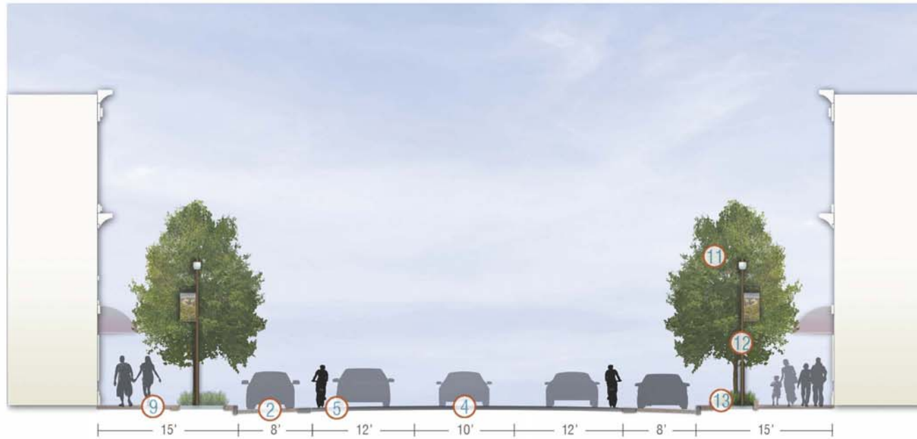
Typical Block Cross Section
