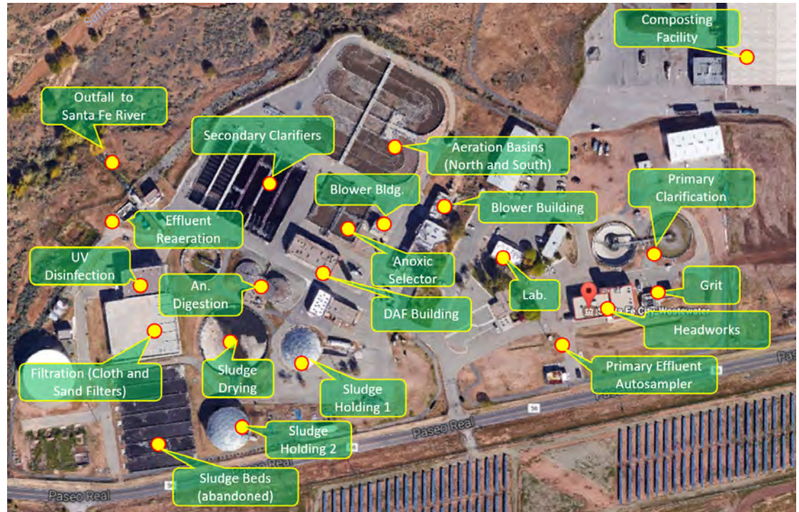
Figure 1.1 Paseo Real WWTP Site Layout
