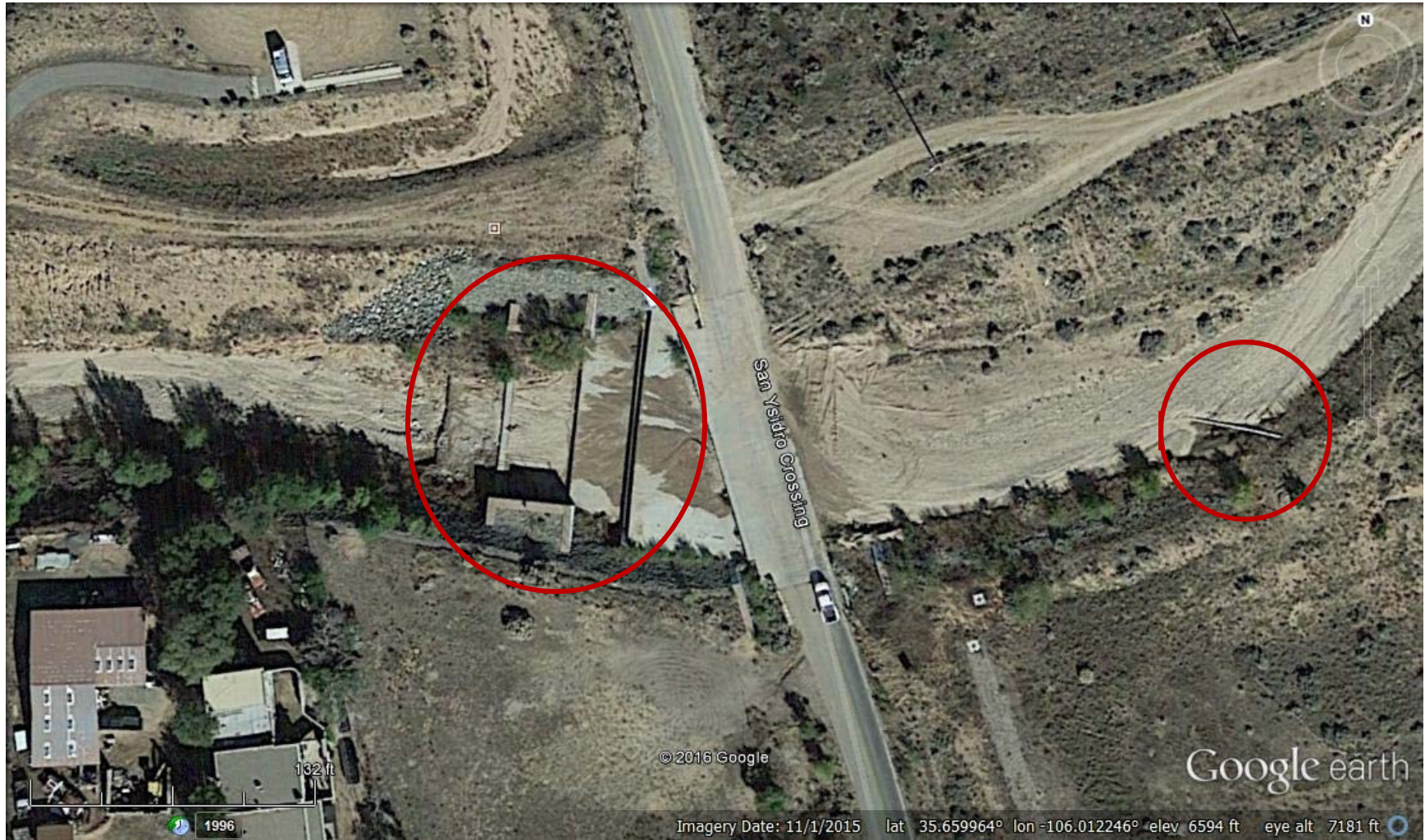
Figure 1. Aerial photograph showing San Ysidro Rd crossing the Santa Fe River. Erosion control features are identified by red circles.
