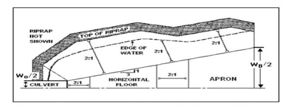
Based on the outlet velocity, the required D50 would be 9 inches and the maximum and minimum acceptable dimensions are:
