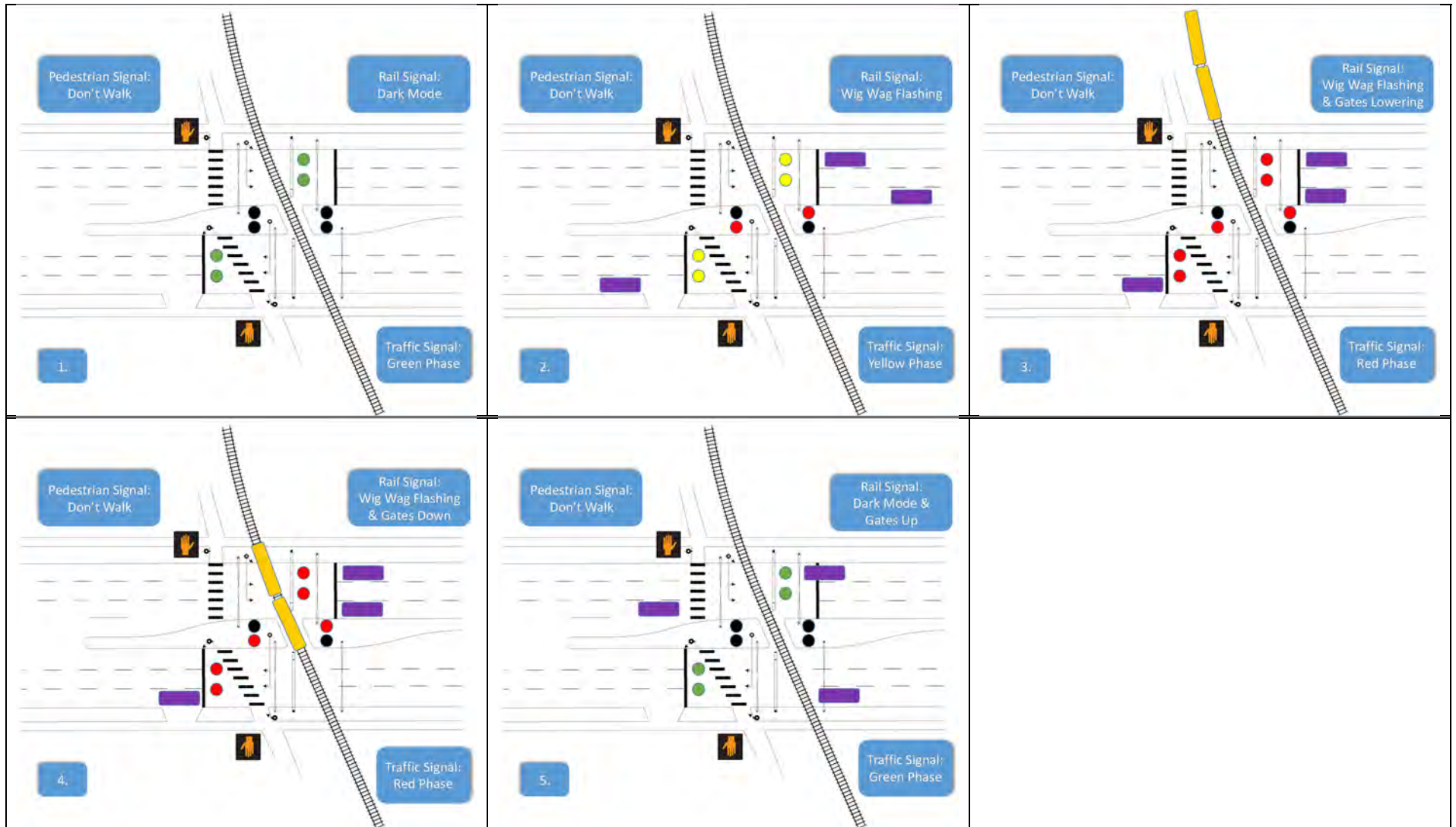
Figure 14. Full Signal Rail Pre-Emption Operation (No Pedestrian Call)
