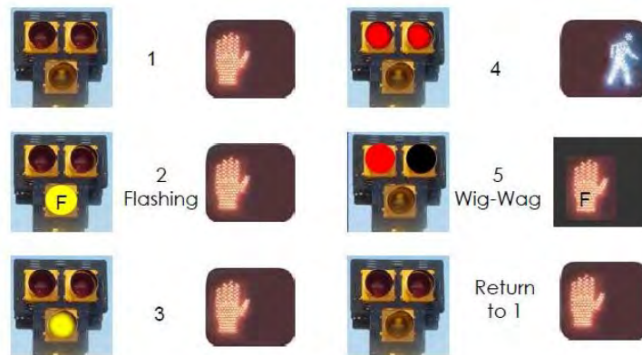
Figure 4.4 PHB Beacon and Pedestrian Signal Indications
