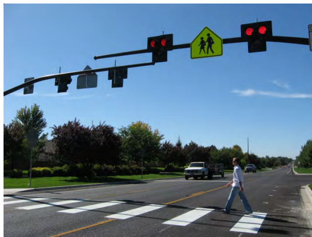
Figure 4.3 PHB Signal Head and Sign Configuration
