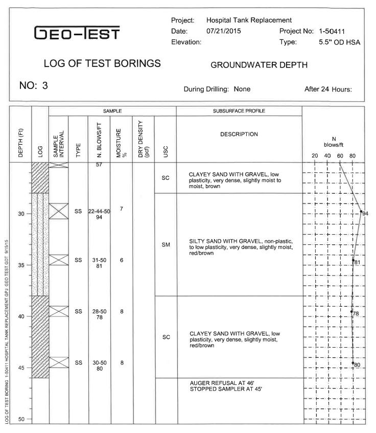
SS - Split Spoon AC - Auger Cuttings UD/SL - Undisturbed Sleeve AMSL - Above Mean Sea Level
